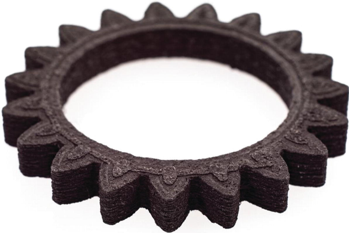
Figure 11-2 A green part made of high-carbon iron (part courtesy of The Virtual Foundry)
