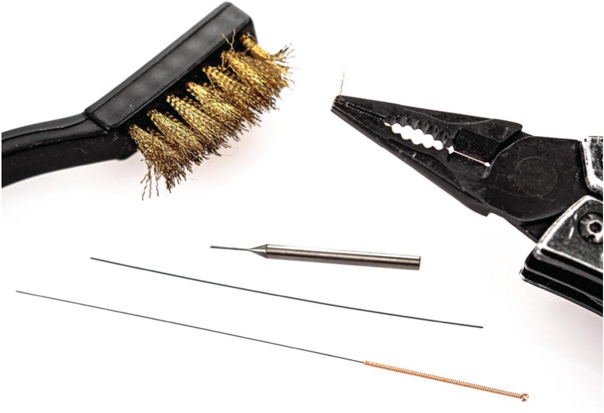
Figure 5-7 Good (and bad) tools for clearing nozzle clogs
