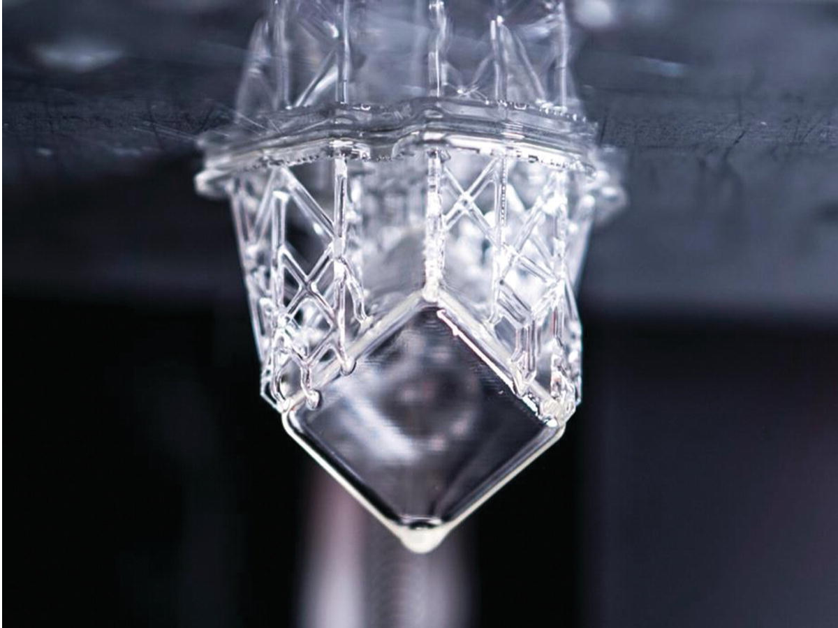
Figure 3-10 A cube created (upside-down) on a resin printer
