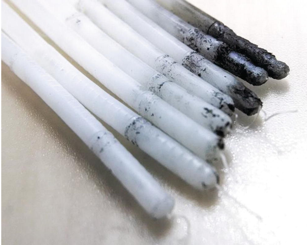
Figure 5-5 Burned residue on cold-pulled filament
