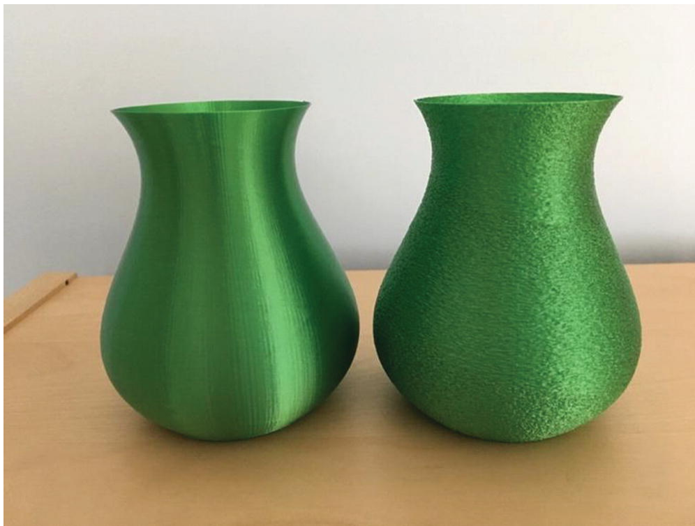
Figure 9-2 Two spiralized vases, the one on the right with “fuzzy skin”
