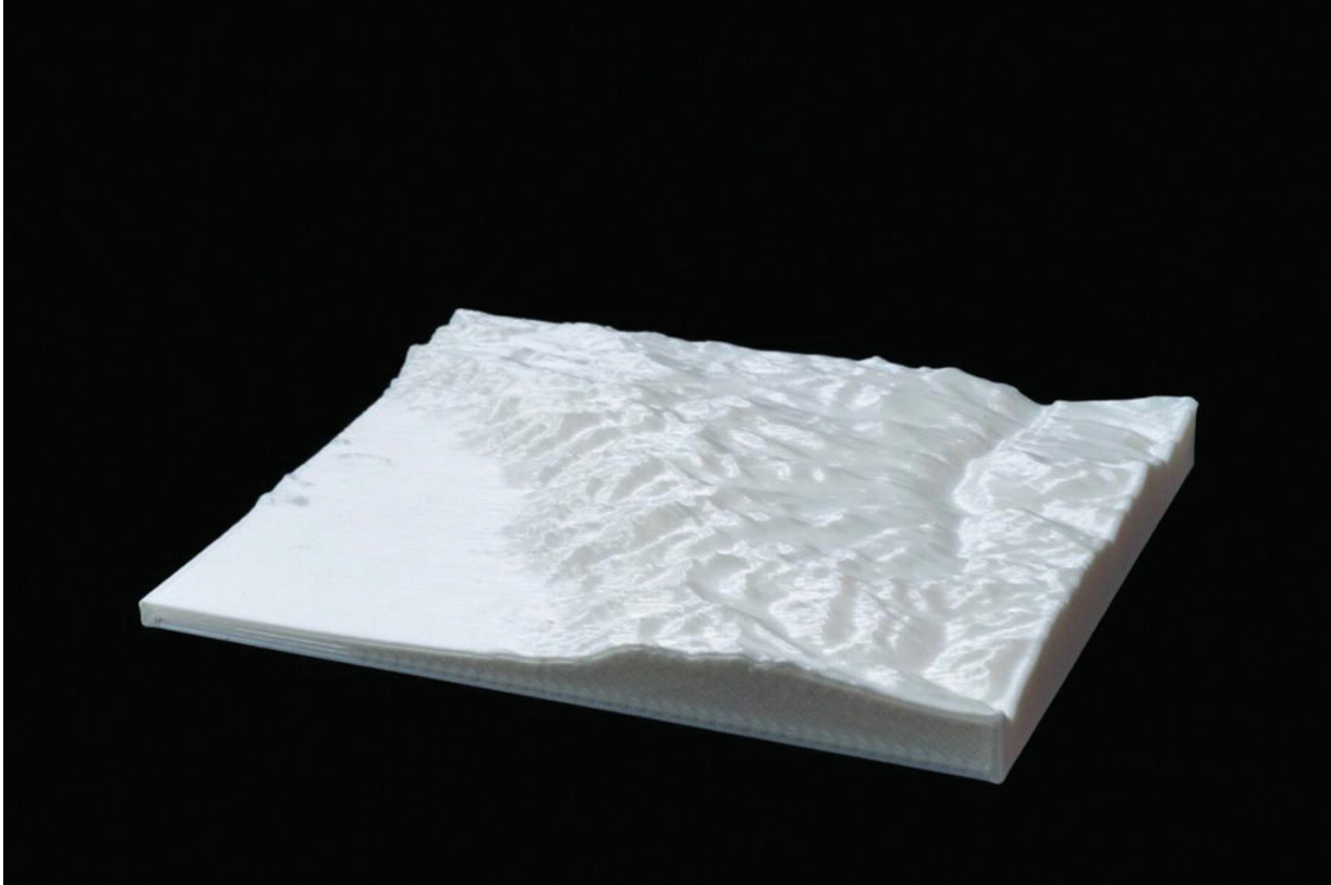
Figure 13-6 Mt. Whitney area, no vertical exaggeration, printed vertically
