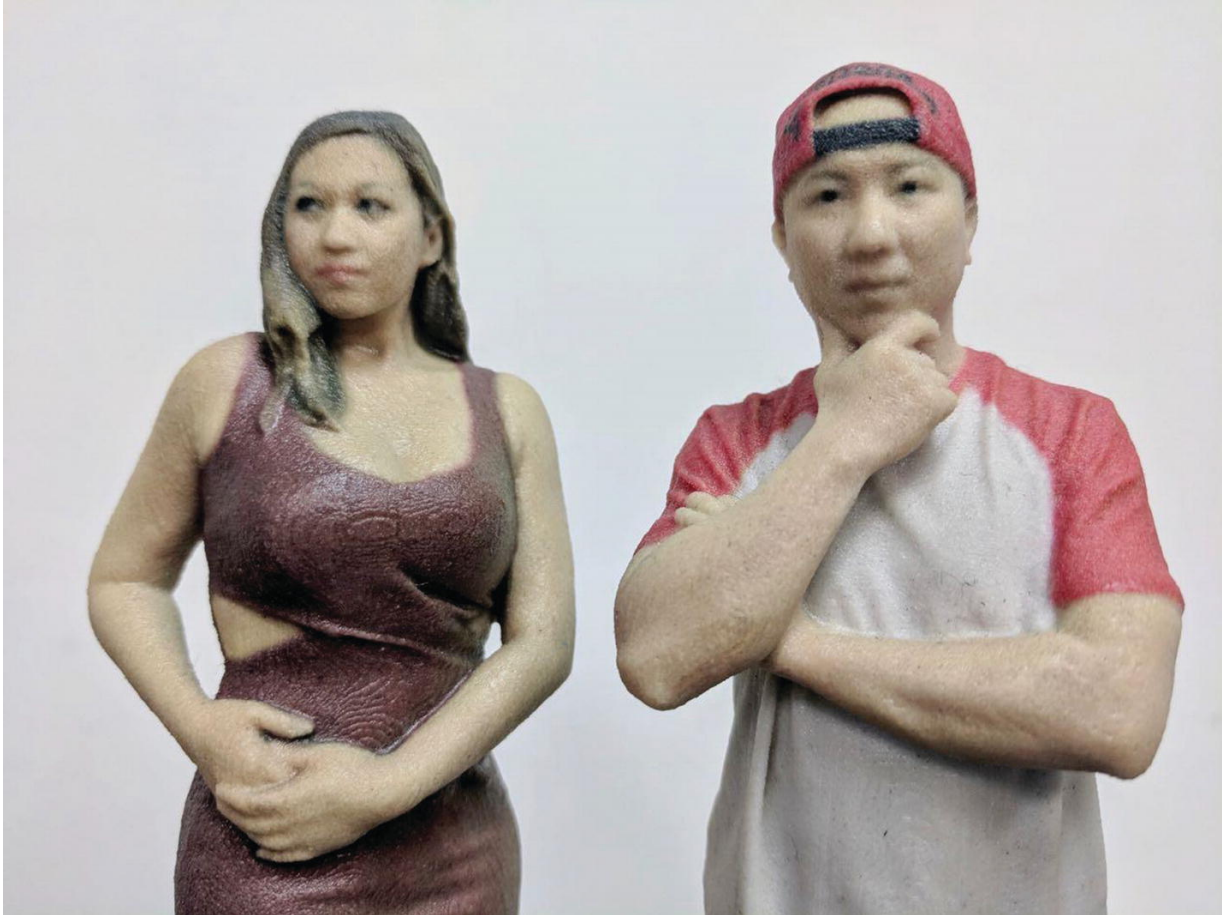
Figure 4-5 Example of full-color binder jet print. Model courtesy of CoKreerate/Will and Jewelyn Co
