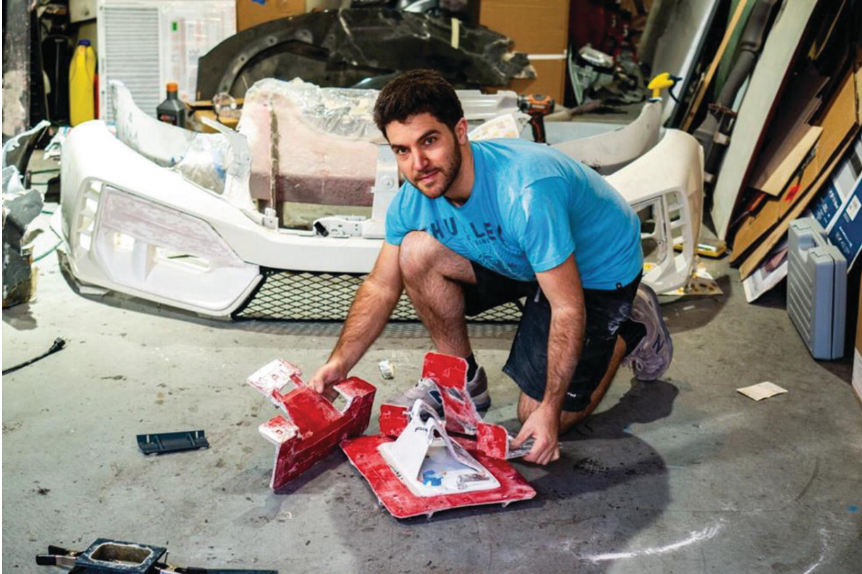
Figure 10-9 Cody Casale shows a mold (red) and molded part (white)
