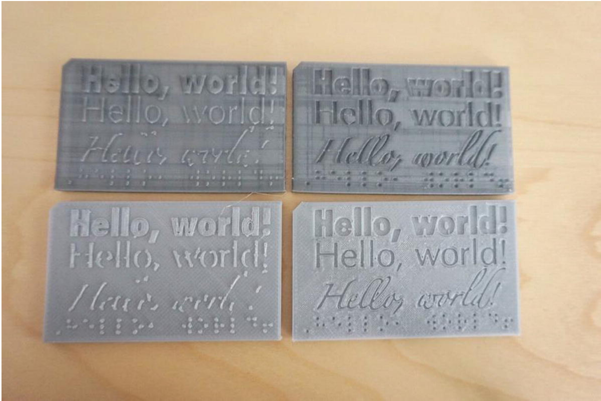
Figure 8-2 Details printed in various orientations
