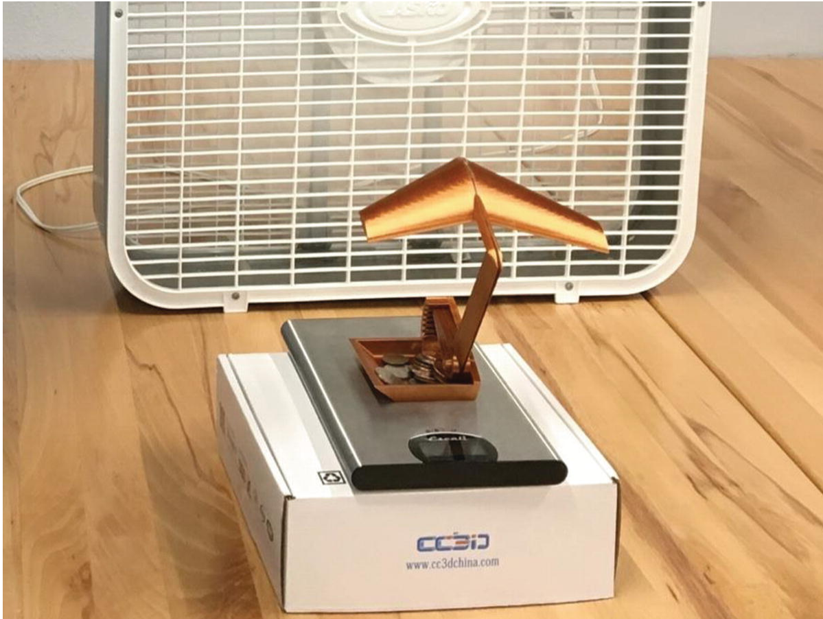
Figure 13-4 The wing's lift being determined
