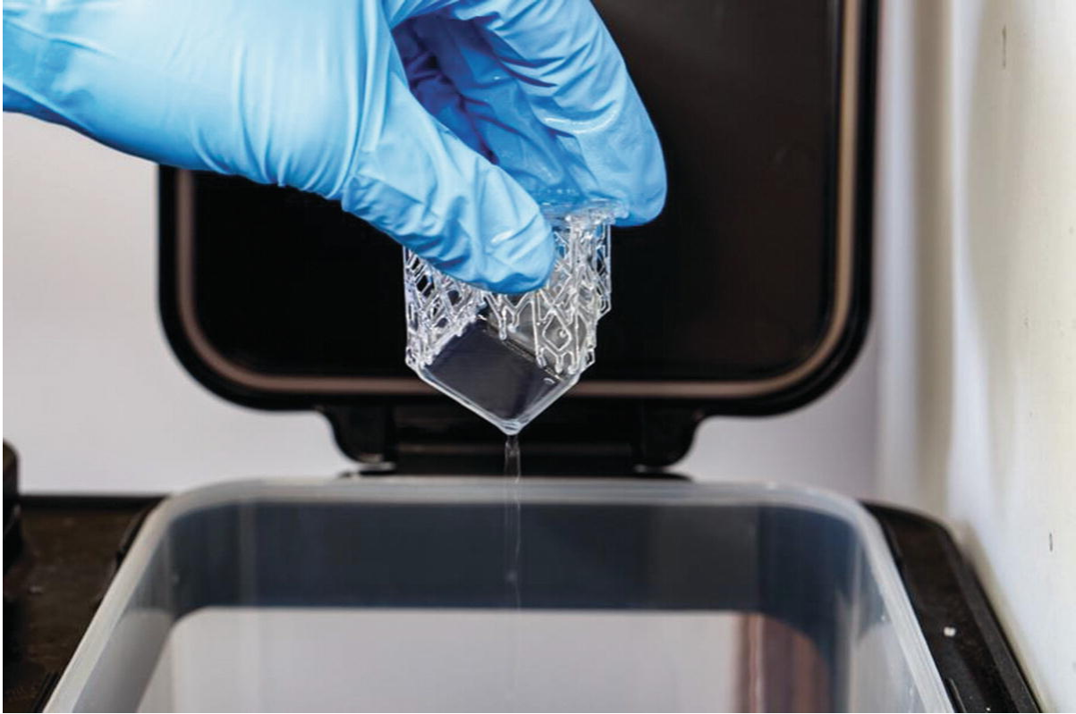
Figure 5-10 A resin print being washed with alcohol in a Formlabs wash station
