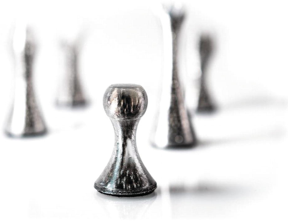
Figure 6-6 Chess pieces printed transparent and filled
