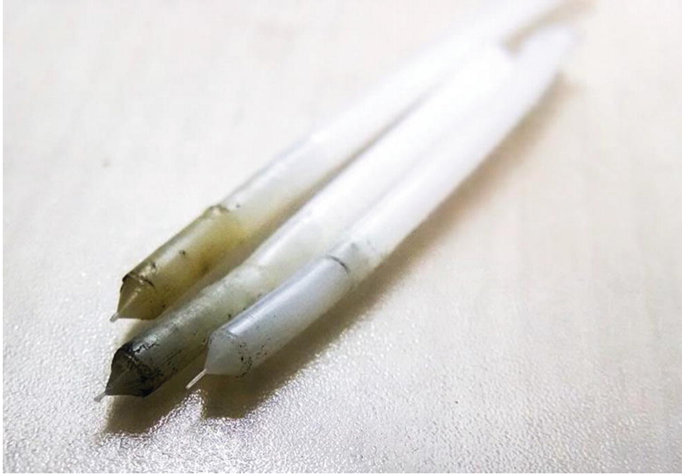
Figure 5-6 Nylon with residue of overheated plastic
