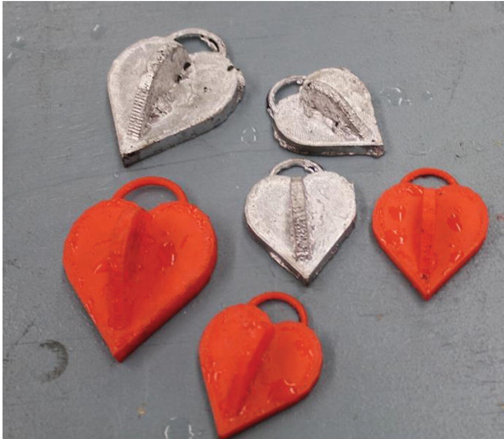
Figure 11-6 Heart patterns and finished aluminum cast pieces
