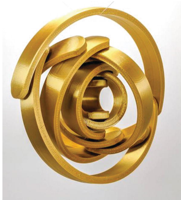
Figure 9-9 The 9-segment Arc Gimbal
