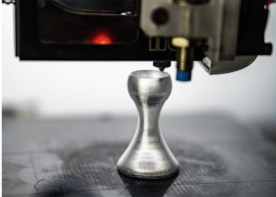
Figure 1-1 A 3D print in progress
