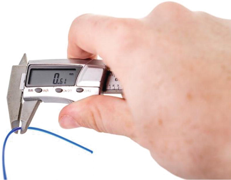
Figure 2-11 Checking filament diameter with a pair of calipers
