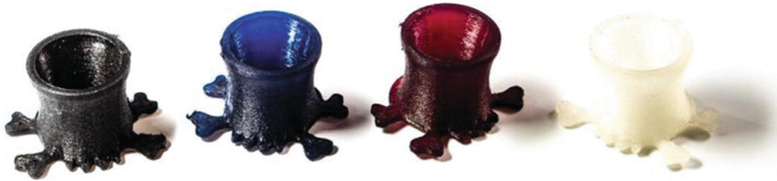
Figure 6-8 Nylon pieces, dyed (three to the left) and undyed (right)
