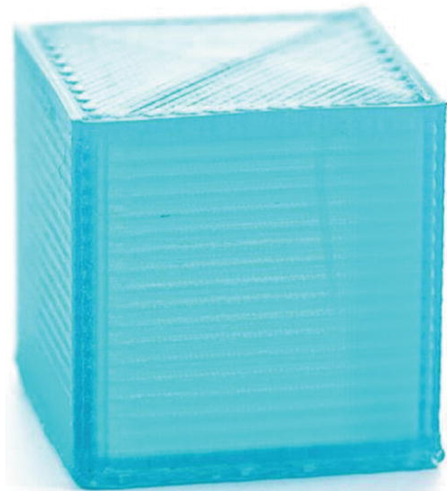
Figure 4-4 Hollow cube printed in PETG
