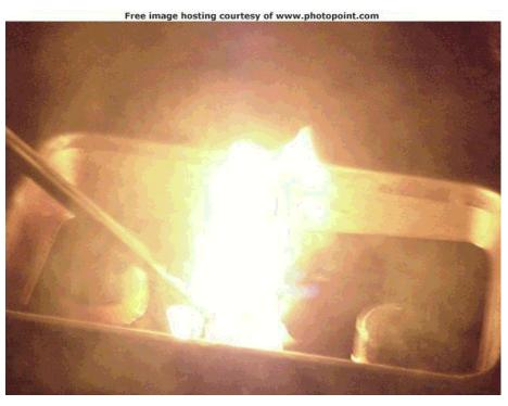
I quenched the blade only putting about 2/3 of the blade in the oil. 2/3 of the cutting edge down and held it there until the flame was gone, about a minute and the slowly placed the rest of the blade in the oil until it was covered and no more smoke.
